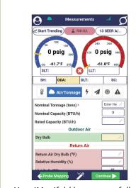
Your iManifold has successfully connected. Select "Probe Mapping" to map wired/wireless probes.
